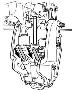
7. Activate the trim-up switch until the tilt rod is fully extended. Unlock the tilt support lever.
