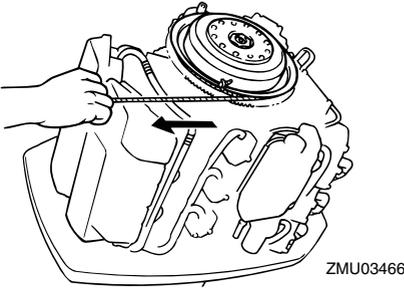
7. Give a strong pull straight out to crank and start the engine. Repeat if necessary.
