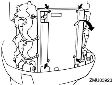
2. Disconnect the yellow cord (emergency circuit) of the CDI unit to return to port.
