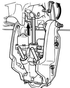
8. Tilt the outboard motor down. Check that the tilt rod and trim rods operate
