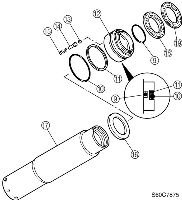
9. Install the backup ring ⑳ and new O-ring ㉑ to the tilt piston ㉒.
