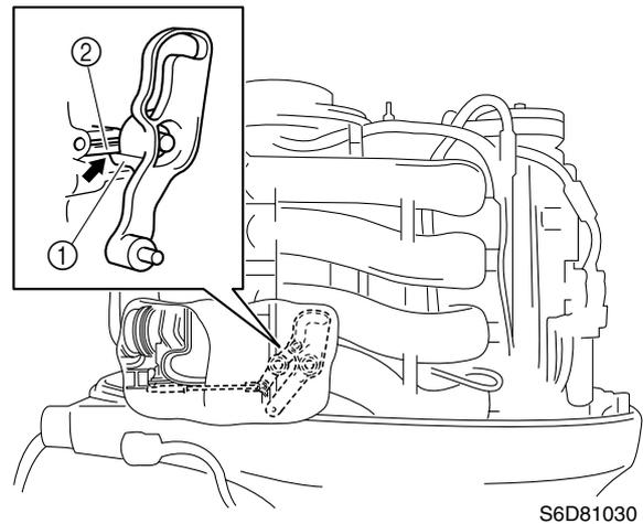
3. Check that the alignment mark ① on the bushing is aligned with the alignment mark ② on the bracket.
