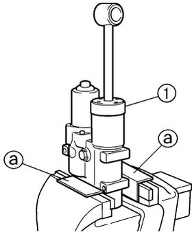
2. Loosen the trim cylinder end screw ②, and then remove it.
