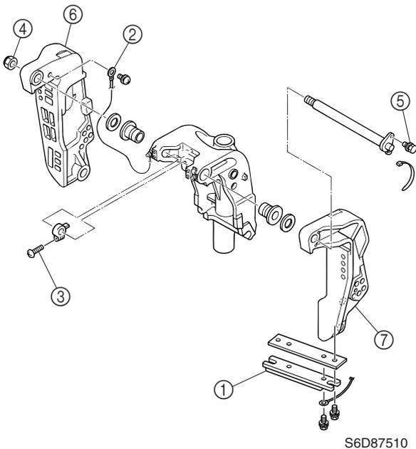
**Installing the clamp brackets**
