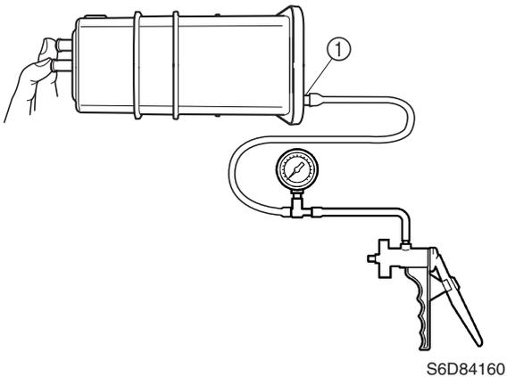
3. Apply the specified positive pressure and check that there is no air leakage. Replace the canister if there is air leakage.
