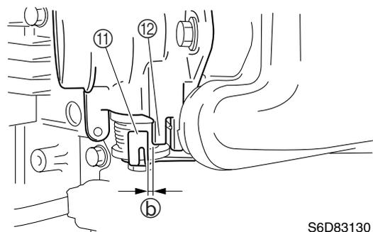
11. Adjust the position of the throttle cable joint until its hole is aligned with the set pin on the throttle cam.
