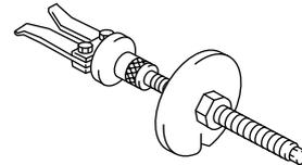
**Bearing outer race puller assembly**
