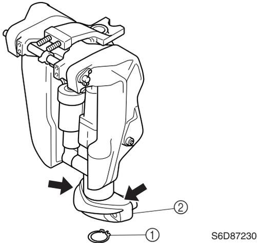
3. Remove the steering arm from the swivel bracket by pulling the arm off the bracket.
