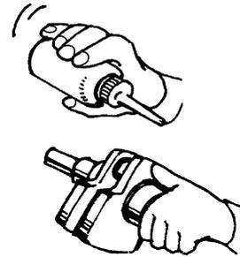
3. Install bearings with the manufacture identification mark in the direction indicated in the installation procedure. In addition, be sure to lubricate the bearings liberally.
