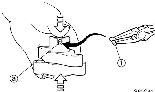
3. Turn fuel pump body 1 ② approximately 90°, and then push down on the plunger several times to make sure that the pin does not come out.
