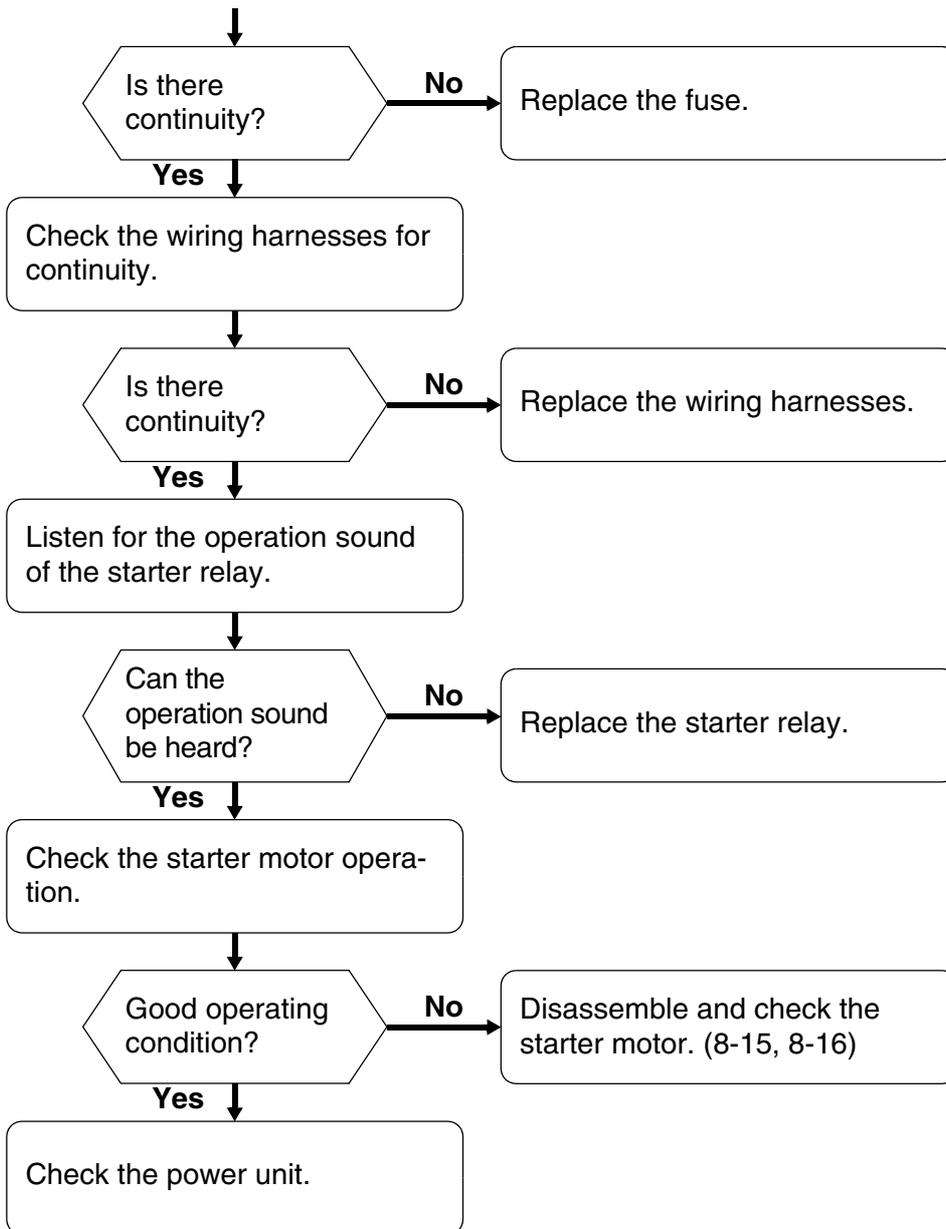
**Symptom: Engine cranks, but will not start (engine stop lanyard switch is operating normally).**
