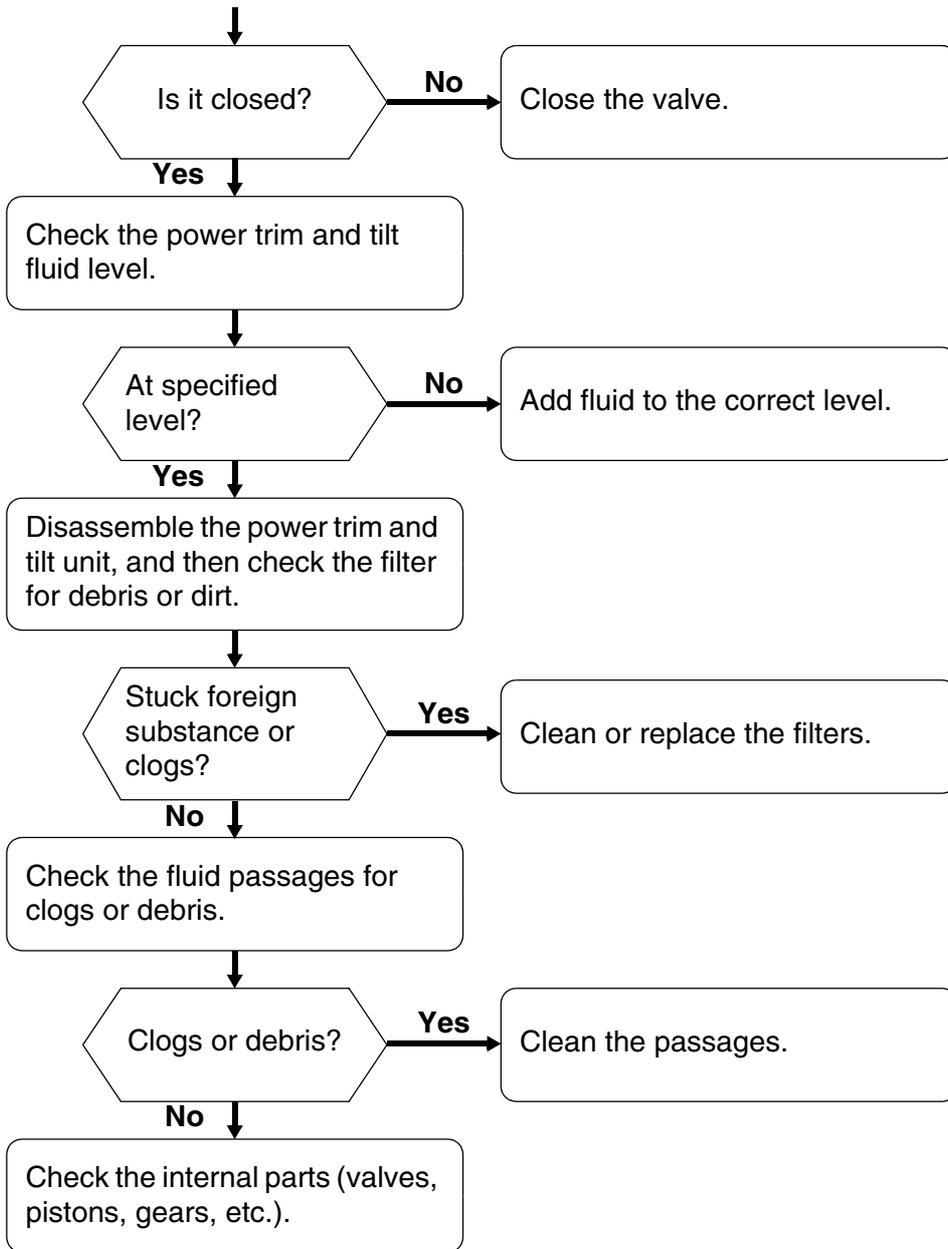
**Symptom: Power trim and tilt unit does not hold the outboard motor up.**
