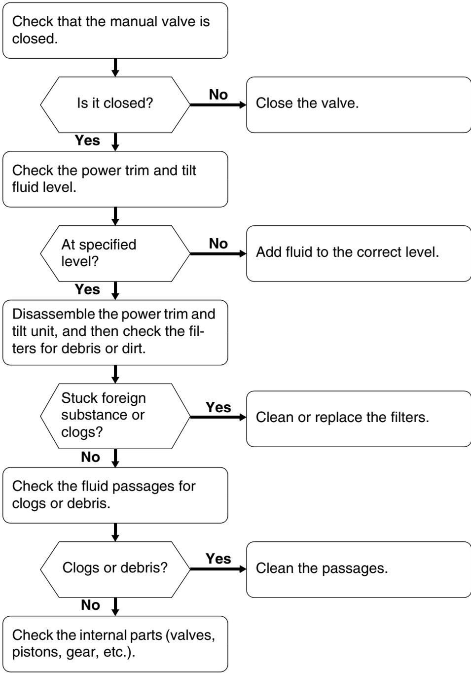
**Symptom: Shift mechanism of the forward gear and reverse gear does not operate properly.**
