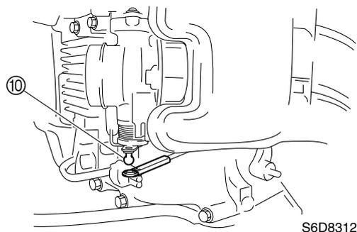
9. Connect the throttle link rod joint, and then tighten the locknut.
