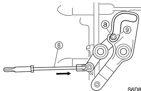
8. Adjust the throttle link rod joint to align its hole with the ball joint ⑩ on the throttle body.
