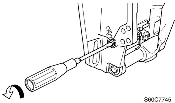
4. Remove the circlips ⑥, then the lower mounting shaft ⑦.
