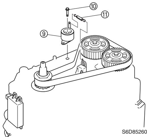
14. Take up the timing belt slack by turning the drive sprocket clockwise at least two full turns.
