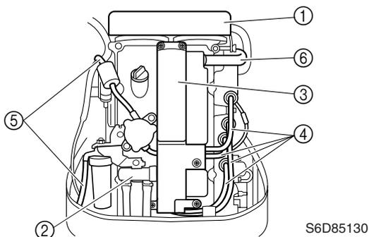
2. Turn the flywheel magnet clockwise and align the "TDC" mark ① on the flywheel magnet with the pointer ②, and check that "▲" marks ③ and ④ on the driven sprockets are aligned.
