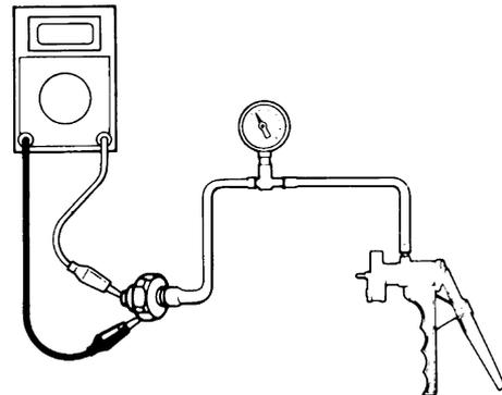
4. Check the oil pressure switch for no continuity at the specified pressure. Replace if there is continuity.
