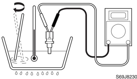
2. Measure the cooling water temperature sensor resistance. Replace if out of specification.
