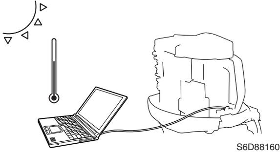
3. If the ambient temperature and the displayed intake air temperature differ by more than  $\pm 5\text{ }^{\circ}\text{C}$  ( $\pm 9\text{ }^{\circ}\text{F}$ ), replace the sensor assembly.
