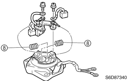
4. Push the brushes into the brush holder, and then install the armature.
