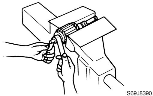
2. Measure the commutator diameter. Replace the armature if below specification.
