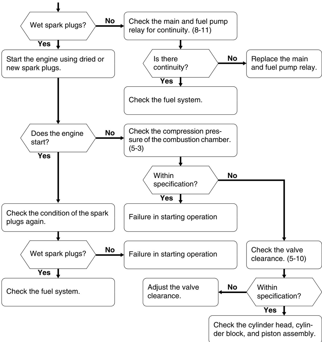
**Symptom: Engine can be started, but does not remain on.**
