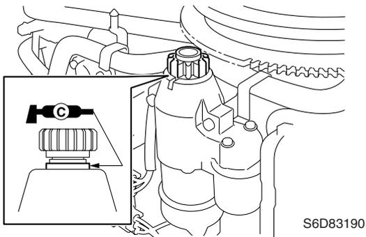
3. Apply corrosion resistant grease to the area shown.
