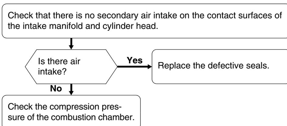
**Symptom: Engine does not accelerate when the throttle is opened quickly.**
