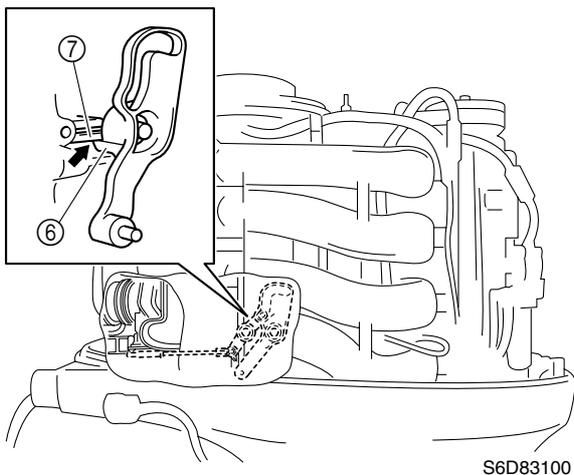
6. Check that the throttle valve fully close.
