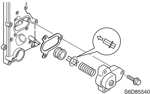
**Installing the exhaust cover**
