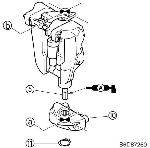
6. Inject grease into the grease nipple until grease comes out from both the upper and lower bushings ③.
